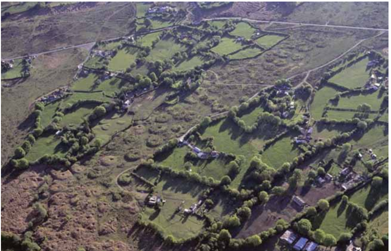
Figure 4.5 Aerial view showing surface evidence of coal extraction using shallow shafts at Titterstone Clee in Shropshire. © Clwyd Powys Trust
